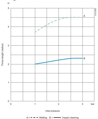
For Clip-on models, the flow rate is increased by approx. 1.5 m<sup>3</sup>/h.
