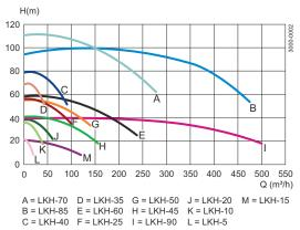
Frequency: 50 Hz Speed (synchr): 3000 rpm
